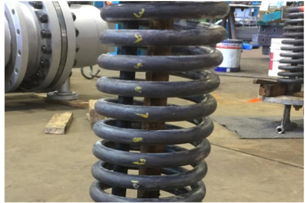
Pipe Coil Fabrication
